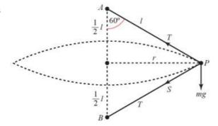
T is the tension in AP and S is the tension in BP. The triangle is equilateral (3 equal sides).
