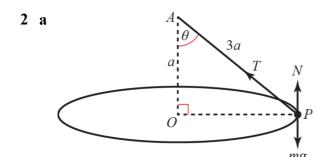
N is the normal reaction of the table on P, T is the tension in the string, and  $\theta$  is the angle between the string and the vertical. Right-angled triangle so
