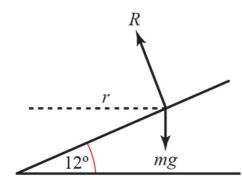
*R* is the normal reaction of the surface on the car. No friction.
