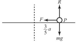
*F* is the force due to friction, *R* is the normal reaction.
